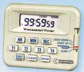
Timer operates on all channels simultaneously. It has five countdown channels, a stopwatch channel, and a time-of-day channel. Counts both up and down to 99 hours, 59 minutes, 59 seconds. Accuracy is 0.01%. Unique thru-zero feature allows counting down, alarming, and counting up. A time-out mode stops the timer for off periods in both up and down timing. T1 through T4 may be started simultaneously
