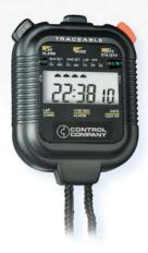
The extra-large display is %-inch for ease in reading. Shows times to 29 minutes, 59 seconds, 99 hundredths. For times exceeding half an hour, the unit automatically goes into an expanded range and times up to 23 hours, 59 minutes, and 59 seconds. As a chronograph, the unit displays time-of-day in hours, minutes, and seconds, AM/PM, date, and day of the week. Also has a time-of-day alarm.
