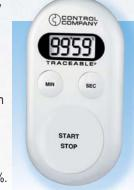
Memory retains last programmed time, eliminating the need to re-enter test times. Alarm may be silenced manually or turns off automatically after 30 seconds.
