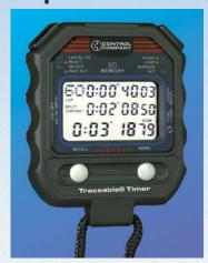
Three-line display simultaneously shows running time, cumulative split, and interval split. Sixty memories recall all splits, display sample numbers 1-60, and show interval split longest, shortest, and average times.
